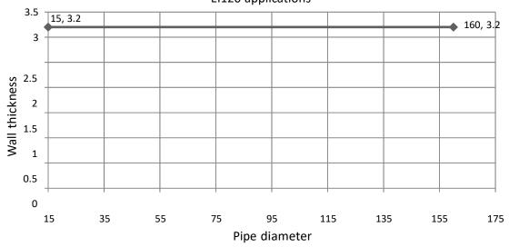
C.1.3 The line graphs below show the coverage of the allowable HDPE (according to EN 1519-1)\* pipe diameters and wall thickness for applications up to El120: (any pipe size variation along the line is covered)
