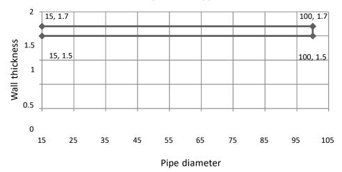
C.3 Field of application for minimum 280mm long Tenmat Firefly 109+ Fire Sleeve – Circular for PVC-U circular ambient pressure extraction and ventilation 'duct' type pipes penetrating fire resistant walls for applications up to El120:
