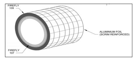
The Firefly 109, 109+ and 109+ LP Fire Sleeve – Circular is available as single sleeve up to 500mm long which can be cut down to suit the intended application. It must be a minimum of 150mm long or longer if the wall is thicker. The Firefly 109, 109+ and 109+LP is delivered in various sizes to fit particular pipe diameters – see table below:
