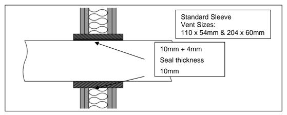
D.6 Field of application for Tenmat Firefly 109+ LP Fire Sleeve – Rectangular (Enhanced Sleeve) for use with a 220mm wide x 90mm high PVC-U rectangular ambient pressure extraction and ventilation 'duct' type pipe penetrating fire resistant walls for applications up to El120:
