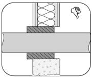
$Rigid \ walls \ must \ comprise \ concrete, \ aerated \ concrete \ or \ masonry \ \geq 650 kg/m^3 \ (Wall \ Type \ A) \ or \ concrete, \ masonry \ \geq 1100 kg/m^3 \ (Wall \ Type \ B)$
